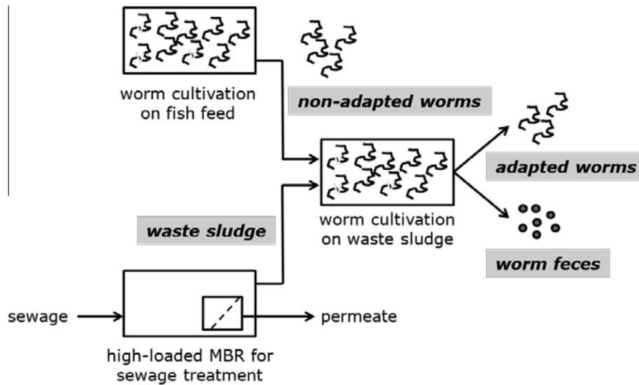
Fig. 1. Experimental set-up to obtain substrates (in gray boxes) for the anaerobic digestion tests.
